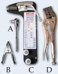
Each cable order comes with a  $\frac{3}{16}$ " Allen Wrench with socket drive (A), a tension gauge (C), a cable gripping pliers (D) and 11 spring clamps (B).
