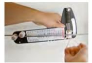
Read the needle position on the scale and refer to the calibration table to determine the tension. The gauge can be left on the cable for "hands free" adjustment.
